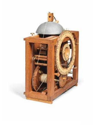
rates of two metals. This, his brass and steel Gridiron coupled to the crucially important adjustable suspension system, the curved cheeks. Fourth: With, once again, all wheel pivots of brass running in bushes of Lignum Vitae the clocks were designed to run indefinitely. This is an overall summary of Harrison's ground breaking innovations with these extraordinary clocks.
