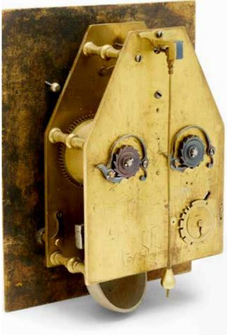
As described by Dawson et al., the movement was originally of twoday duration and later converted to eight days by reversing the barrels and inserting intermediate wheels. The clock is significant because very few short duration clocks have survived from this period. As a practical matter, eight day clocks would have been favored over ones of shorter duration.
